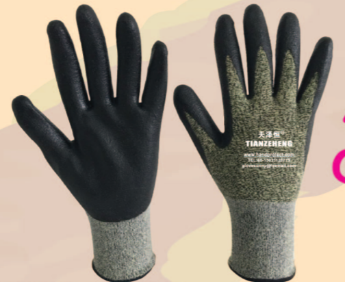
ITEM NO.KVNR708B 13 Gauge Aramid +Glass Fiber+Modacrylic Liner Neoprene Foam Coated ARC Flash 10 cal/cm 2
