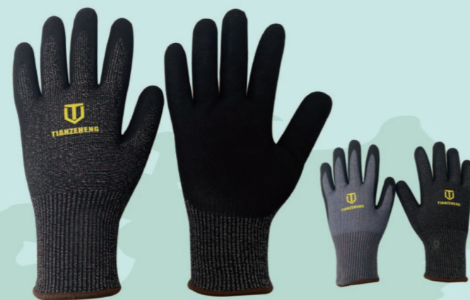
SMDQ408B 13G Synthetic Anti-cut Liner Sandy Nitrile Palm Coated Level :C EN 388 ANSI CUT A3 4543C
